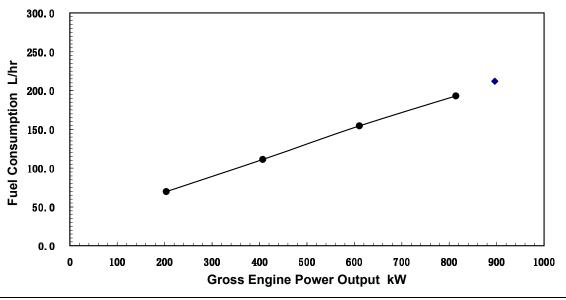
**Rating Conditions:** Ratings are in accordance with ISO-3046 reference conditions; air pressure at 100 kPa (29.61.in Hg.), air temperature 25°C (77°F), and 30% relative humidity. The fuel consumption data is based on GB252 No.0 diesel fuel (No. 2 diesel fuel in U.S.) weight at 0.85 kg/litre (7.1 lb/U.S. gal).
