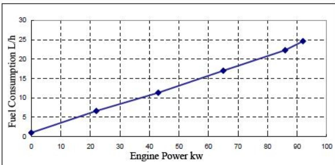
Performance data obtain under normal conditions, according to GB/T18297 test conditions
